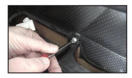
9. Remove triangular plastic cover at "hinge end" (covering the mirror bolts). You may need to wedge a flat screw driver between the cover and the door frame to unclip the small plug which keeps the cover in place.
