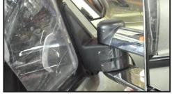
15. Screw in the top bolt first (initially not too tight) then the others. Then tighten all bolts.
