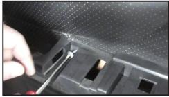
5. Remove the screw at the bottom of the handle section of the electrical control panel.
