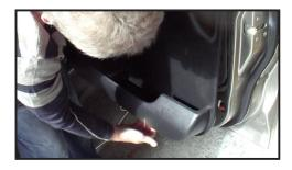
The next procedure is to remove the existing mirror and to install the ORA XL. *It may be helpful to have another person assist in holding the mirrors whilst they are being detached and installed.*
