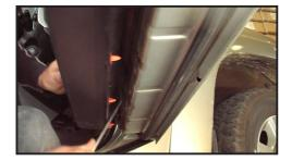
11. Once all the plugs have been detached gently tap the base of the panel until the whole panel separates from the door frame.
