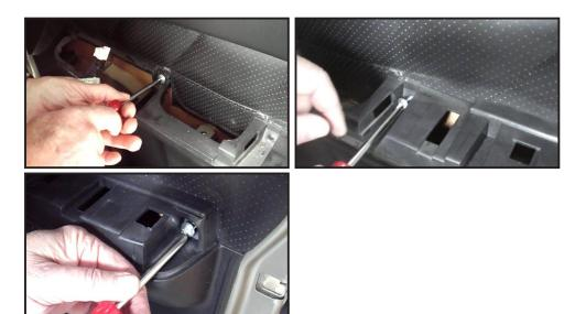
19. Replace the control panel electrical plug. Then put the electrical control panel back in position.
