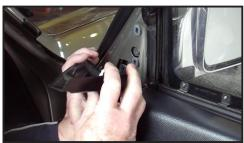
10. The door panel connects to the door with several hidden plastic plugs that run along the base and up each sides. The plugs at the base of the door are located beside indents in the metal frame. Locate these indents and gently prise the panel away from the frame with a long flat screw driver. Continue pulling the panel up the sides of the door until all plugs have unclipped.
