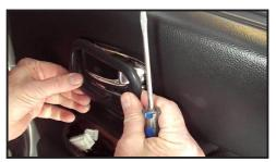
3. Remove arm rest cover. You should be able to do this by hand. Grip the "latch end" of the cover and lift. Use a flat screw driver if it doesn't come away easily.
