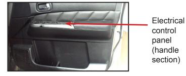
6. Lift out the electrical control panel from the "hinge end" first. This can be done by hand, although a flat screw driver may help unclip that end.
