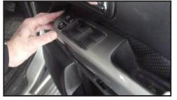
20. Replace the vertical screw that holds the electrical control panel in position.
