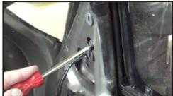
14. Thread through the ORA XL mirror electrical cable. Then position the new mirror in place ensuring that the rubber seal is flush and in position.
