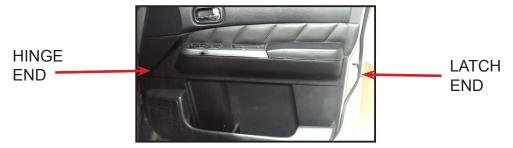
Removing the door panel from the door frame.
