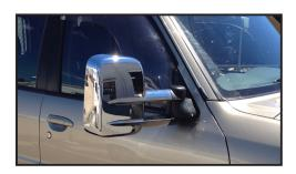
The Mirrors are preset to the optimum angle for viewing from the driver's position. However they will fold in if you accidentally strike an object.
