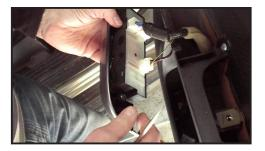
7. Remove electrical plug behind the electrical controls. There may be 2 electrical plugs on the driver's side. The small plug is removed by pressing the small tag. The other plug may need to be wedged out with a small flat screw driver.
