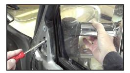
16. Connect electrical plug ends. Then check that the electrical mirror buttons work. The larger top section of the mirror should move left/right/up/down as your standard mirror did. The bottom mirror is manually adjusted. Replace the clear plastic dust cover.
