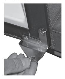
Unscrew the three screws and remove lower hinge. Save the screws.
