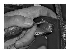
11. Remove the travel catch by unscrewing the two screws. (Save screws and catch.) Two types of screws are used. Make a note of their position in order to install these correctly when reinstalling.
