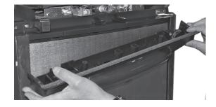
2. Use a socket wrench to loosen the upper hinge pin. Remove pin and save for later use.
