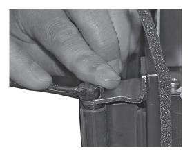
3. Lift the door off the lower hinge pin.
