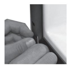
8. Locate the new hinge. Insert hinge pin into hinge hole. Secure the hinge with the three screws removed earlier.
