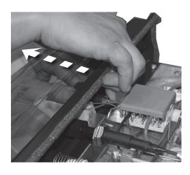
Disengage the seal strips from panel.
