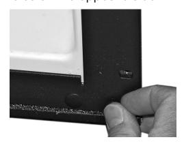
10. Remove upper hinge by unscrewing the two screws. Save screws.
