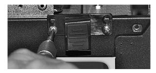
13. Install the new hinge. Fasten with two screws.
