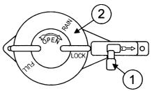
To Close: Rotate control (2) counterclockwise.
